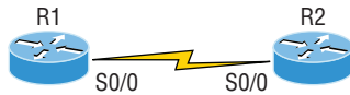
FIGURE 7.24 By looking at R1, the show controllers command reveals that R1 and R2 can't communicate.
